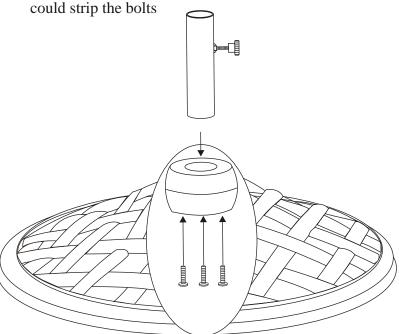
Step 3: Your umbrella base is now ready for use. Carefully guide the umbrella pole through the hole in the center of the table, and if applicable, through the hole in the table connector ring, and then into the base. Using the screw already in place in the extension pole, turn until your umbrella pole is secure in the extension pole.
