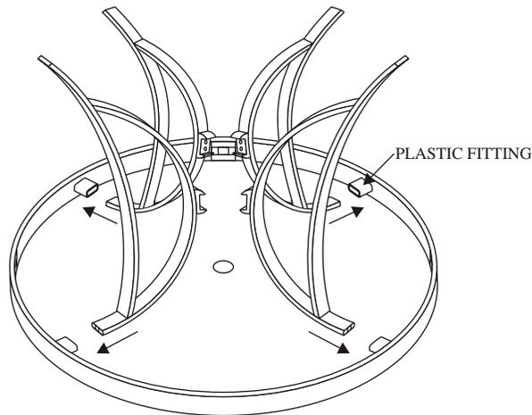
**Step 3:** Attach one leg to the leg connector bracket using two bolts. Add a metal plate to the bolts and guide through the inside of the connector bracket into the fixed nuts inside of the table leg. Hand tighten three or four revolutions only. **Important note: Hand tighten only as some adjustments may be necessary to ensure legs are properly aligned.** Repeat procedure on other three legs, adjusting as necessary to ensure the legs are properly aligned.
