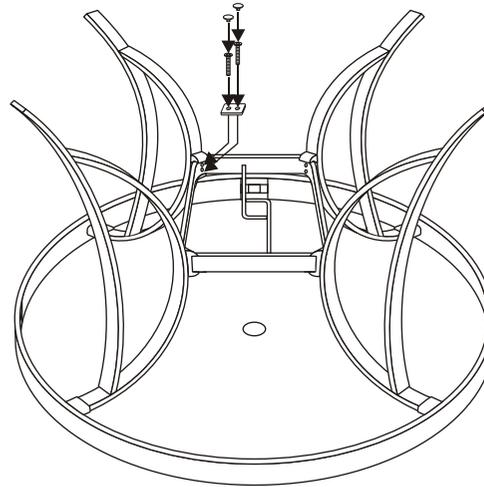
**Step 4:** At this time tighten all bolts using the Hex Bolt Driver provided. Important note: each bolt should be tightened a few revolutions at a time. We recommend working in a cross corner "X" fashion, alternating between bolts. This will tighten the frame evenly by placing equal pressure on all bolt joints. **Do not over tighten.** Cover all bolts with PVC bolt covers provided.
